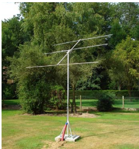
Figure 8 : Antenne Yagi 3 éléments.
